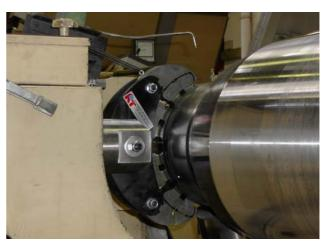
**RON-MASTER**<sup>™</sup> is equipped with the unique supporting shoe. It is based on the special theory of multi-point centering. Such supporting shoe can increase accuracy of rotation dramatically. It decreases the neck's center runout for 60–75% in comparison to the rigid steady rest. As result **RON-MASTER**<sup>™</sup> provides roundness of the ground surface in 2.5-4 times better than roundness of the neck was.
